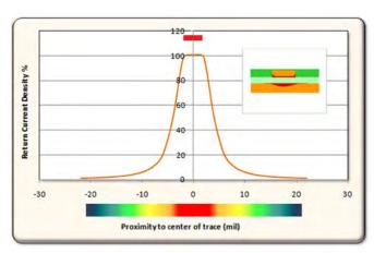
Figure 2: Microstrip return current density.
