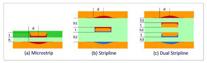
Figure 5: (a) Microstrip, (b) stripline, and (c) dual stripline configurations.
