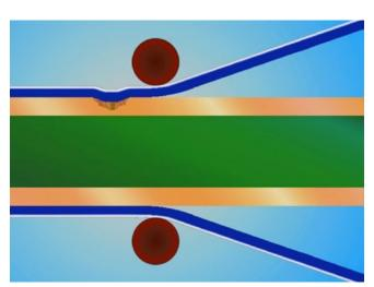
Figure 1: Hot roll lamination; depression in foil may prevent resist adhesion.
