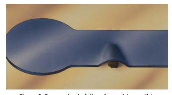
Figure 2: Depression in foil surface with possible resist adhesion issue.
