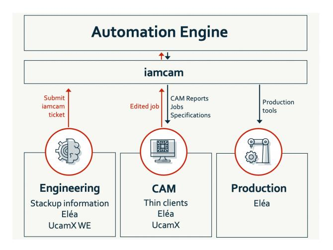
cam ticket defined specific requirements such as minimum annular rings and clearances, depending on IPC classification, copper weights, layer count, etc. And if all the requirements were not quite reached but close, it listed the type and scale of edits that the system was approved to make without having to refer the job back to the customer.
