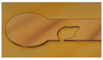
Figure 3: After etching and resist stripping, copper etched away where the resist did not adhere. (Source: IPC)
