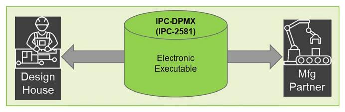
Figure 2: IPC-2581 Rev C Solution improves the DFX processing and communication by creating an open standardized format using XML with tags.
