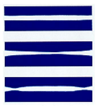
Figure 4: A schematic of the rolls (top and bottom). The top shows good condition. The middle and bottom pairs show bow and other deterioration. (Source: Tim Blair)
