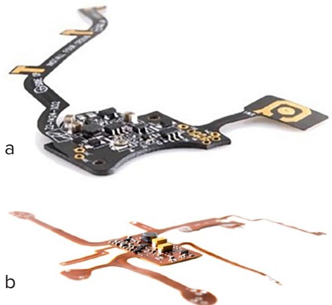
Figure 3: a) Rigidized 3-layer black Kapton with FR-4 stiffener; b) Rigidized 3-layer with FR-4 stiffener.
