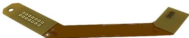
Figure 5: Plated through-holes on the back side of a flex.
